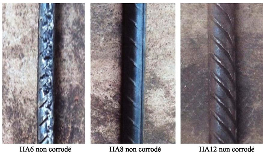
**Figure 3.** Standard uncorroded reinforcements in HA steel.
