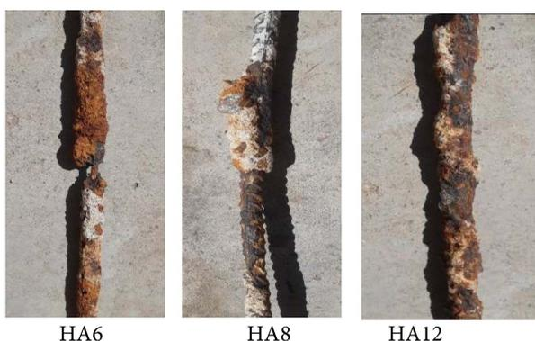
**Figure 2.** Samples of the reinforcements taken showing a layer of rust.
