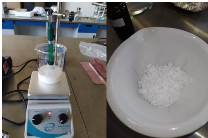
Figure 4. Preparation of nanoparticles from Aloe vera extract.
