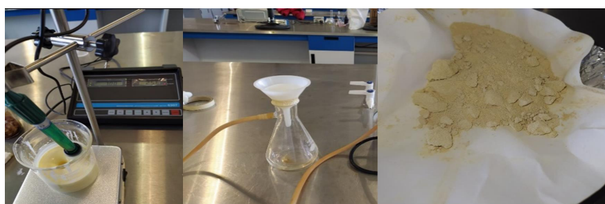
Figure 5. Preparation of nanoparticles using orange peel extract.
