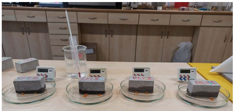
Figure 3. Experimental set-up for the capillary absorption measurements at the building materials. Laboratory of the University of Cyprus.
