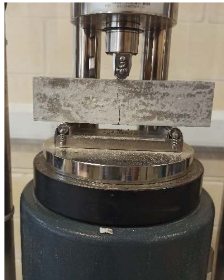
Figure 2. Three-point bending test following EN 12390-5 [20]: (a) schematic representation; and (b) flexure test set-up.
