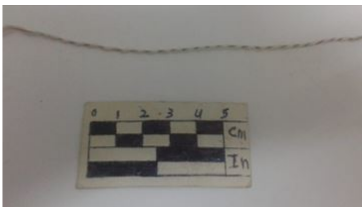
Figure 11. The metallic thread after the artificial aging process.
