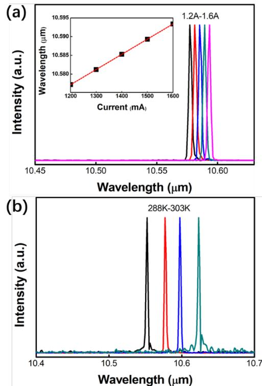
**Figure 2.** (a) CW lasing spectra at a different injection current from 1.2 to 1.6 A with a step of 0.1 A. The inset shows the linear-fit tuning characteristics of the lasing wavelength with electrical power for the same device. (b) CW emitting spectrum of QCL at different heat sink temperature between 288 and 303 K.
