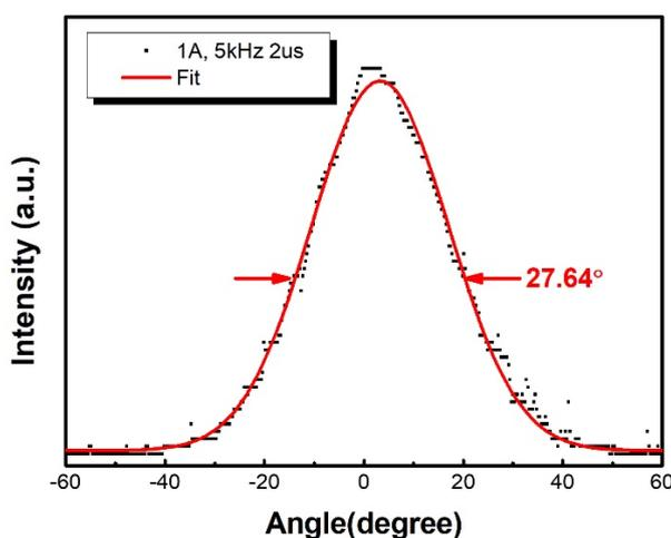
**Figure 4.** Measured lateral far-field radiation patterns for the devices at pulsed driving currents of 1 A under 5 kHz repetition frequency and 1% duty circle, the dot is the measurement and the red dashed line is the result fitted with the Gauss function.
