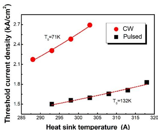
**Figure 3.** Threshold current density as a function of heat sink temperature in CW and pulsed mode of a 4-mm-long and 13- $\mu\text{m}$ -wide LWIR QCL. The red dashed line is fitted with the exponential function  $J_{th} = J_0 \exp(T/T_0)$ .
