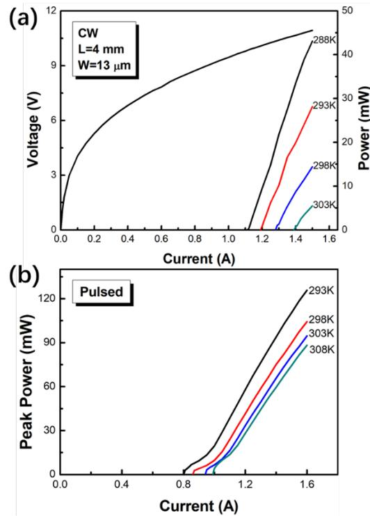
**Figure 1.** (a) Output optical power versus injection current of a 13  $\mu\text{m}$ -wide and 4-mm long device in CW mode at different heat sink temperatures between 288 and 303 K along with V-I curves at 288 K. (b) Peak power of the laser changes with heat sink temperatures at the repetition frequency of 5 kHz and a pulse width of 2  $\mu\text{s}$ .
