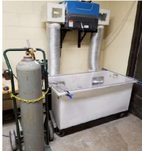
Figure 2. Accelerated carbonation setup.
