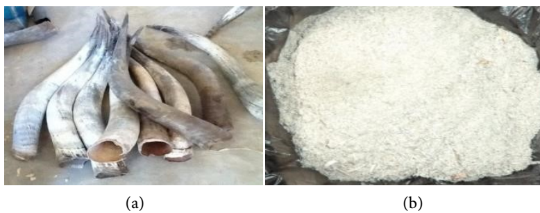
Figure 2. (a) Beef horn sheaths; (b) fine sheath particles almost ready to be used.
