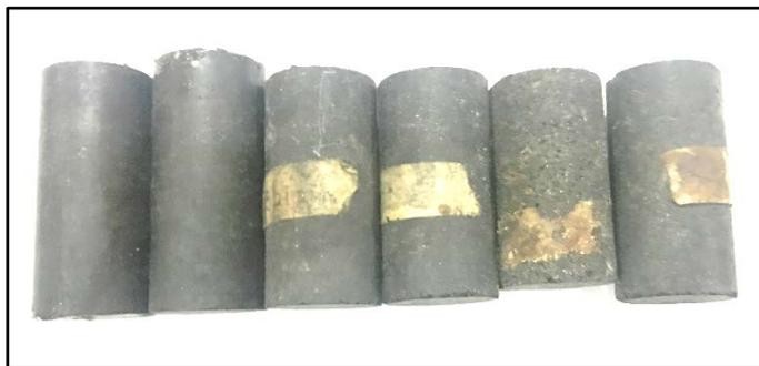
**Figure 1.** The produced GP-resin ETE electrodes.
