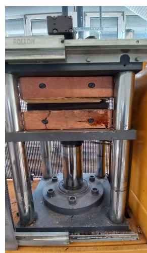
Figure 6. Sanitary pad with wooden mold placed in hot pressing machine.
