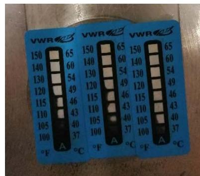
**Figure 5.** (a) Scheme of the position of the temperature sensors on the substrate; (b) temperature indicator strips after plasma exposure.
