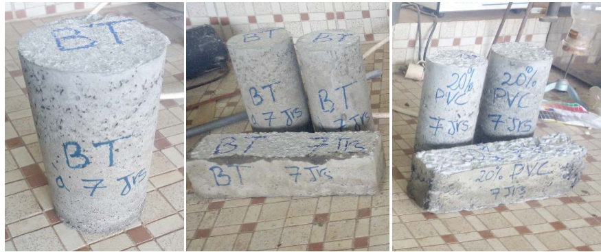
Figure 3. Cylindrical and prismatic specimens.
