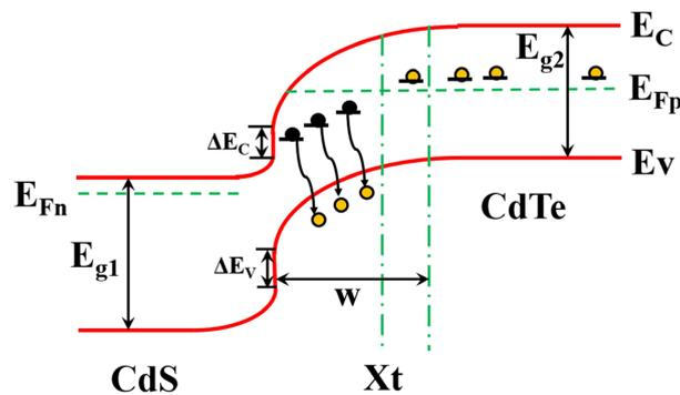
**Figure 9.** Energy band diagram of solar cell for reverse bias conditions (at  $\tau = \infty$ ) consisting of a CdTe absorber with interface states and deep levels. The symbols represent their usual meanings.
