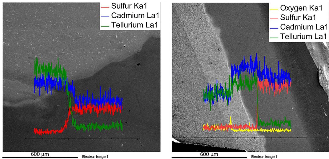
**Figure 4.** EDX line scan of cross section of Cd, S, Te and O profile, CdS/CdTe, (left), CdS/CdO/CdTe (right).
