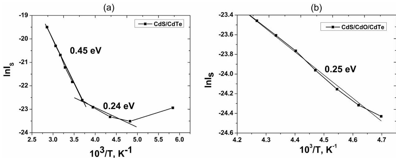
**Figure 7.** The saturation current density dependency on  $1000/T$  for CdS/CdTe (a) and for CdS/CdO/CdTe devices (b).
