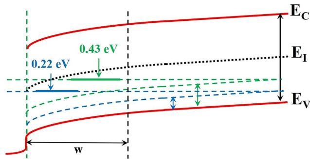
**Figure 12.** Schematic of the assumed energy diagram of CdTe layer in the CdS/CdTe heterojunction device.
