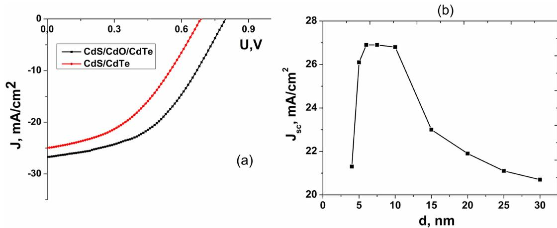
**Figure 5.** The J-V characteristics of the CdS/CdTe and CdS/CdO/CdTe heterostructures under  $100 \text{ mW/cm}^2$ , 300 K (a) and dependence of  $J_{sc}$  in function of the CdO insulating layer thickness (b).
