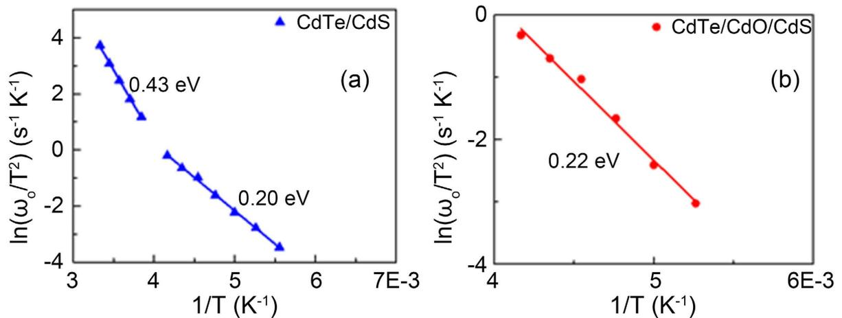
**Figure 11.** The Arrhenius plot of the  $\ln(\omega_0/T^2)$  versus  $1000/T$  of CdS/CdTe thin film solar cells, without (a) and with a CdO layer (b) at the interface.
