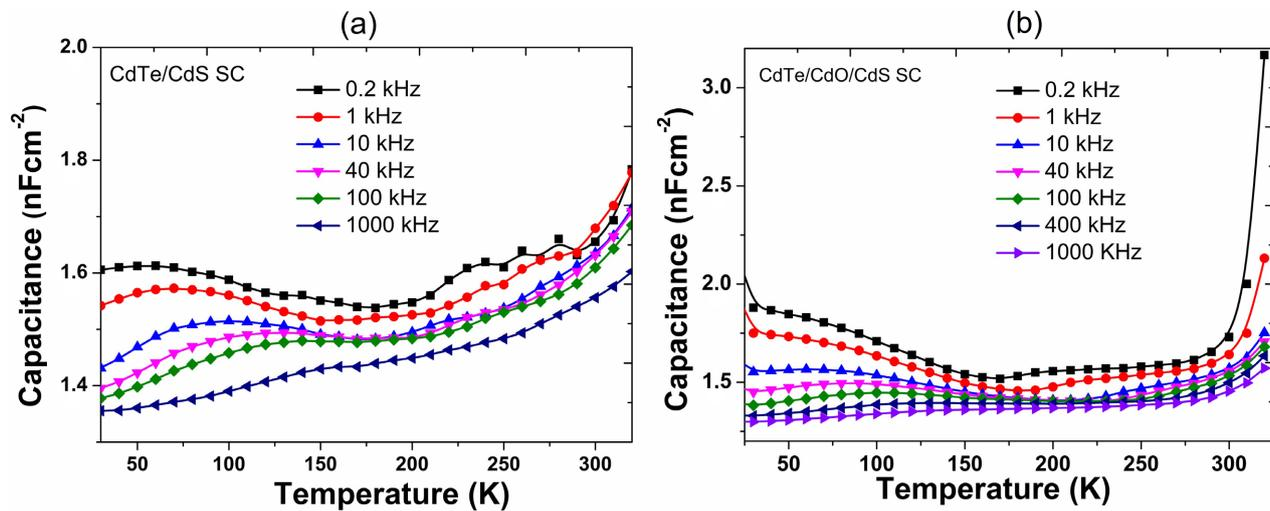
**Figure 10.** C-T-f curves of CdTe/CdS thin film solar cell, without (a) and with a CdO layer (b) at the interface between CdTe and CdS.
