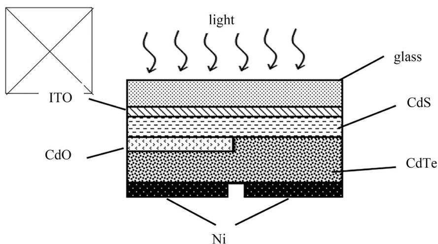
**Figure 1.** The cross section of a CdS/CdTe photovoltaic device with and without interfacial CdO nanolayer.
