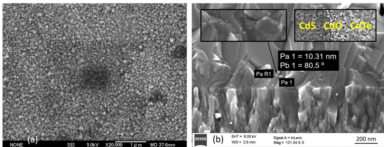
**Figure 3.** The SEM image of CdO deposited on CdS (a) thin film and cross-section image of TCO/CdS/CdO/CdTe structure (b). The insets in cross-section image of a CdS/CdO/CdTe heterostructure present the non-uniform accumulation of CdO at the interface.
