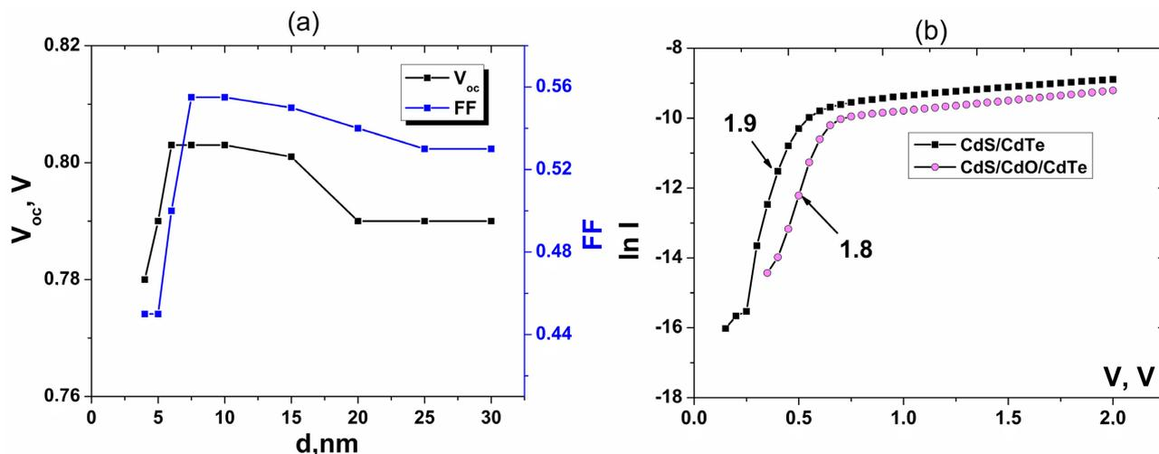
**Figure 6.** Dependencies of  $V_{oc}$ , FF parameters of CdS/CdO/CdTe devices in function of the CdO insulating layer thickness (a) and the dark I-V characteristics of CdS/CdTe and CdS/CdO/CdTe heterojunctions at room temperature (b).
