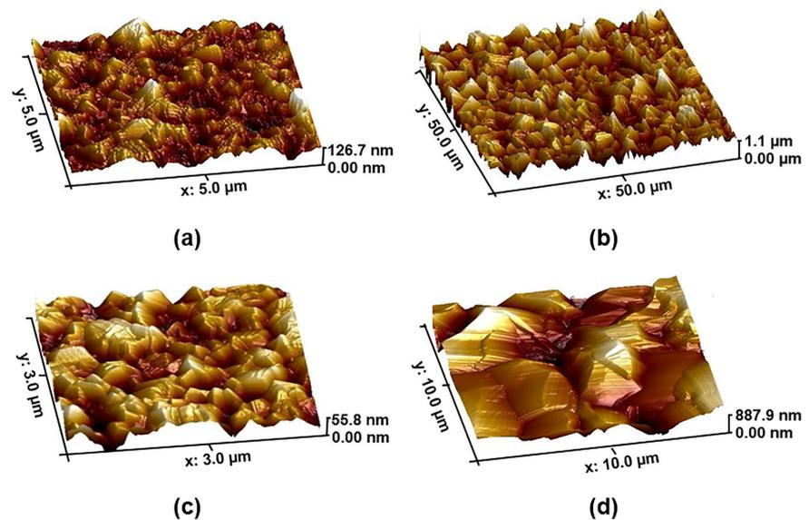
**Figure 2.** The AFM topography of CdS thin film surfaces on glass substrate (a), on CdTe thin film (b) and on CdTe/CdO interface (c). The AFM of CdO nanolayer surface deposited on CdS thin film (d).
