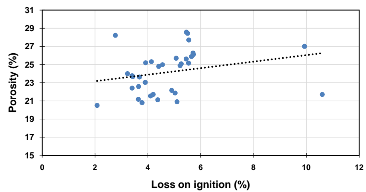
Figure 10. Effect of CBA wt% increasing on the porosity and the loss on ignition of some specimen.
