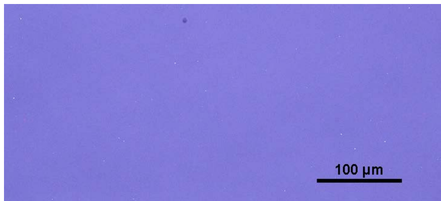
Figure 1. Infrared transmission image of part of the CdZnTeSe wafer. It shows that the wafer is almost free with Te inclusions, and there are no sub-grain boundary networks.
