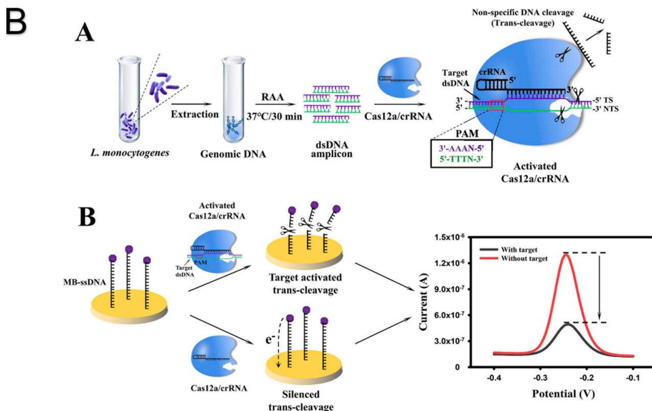
**Figure 5.** Principles of foodborne pathogen detection by electrochemical sensors (A) An electrochemical biosensor for the highly sensitive detection of *Staphylococcus aureus* based on SRCA-CRISPR/Cas12a [53]; (B) An ultrasensitive CRISPR/Cas12a based electrochemical biosensor for *Listeria monocytogenes* detection [54].
