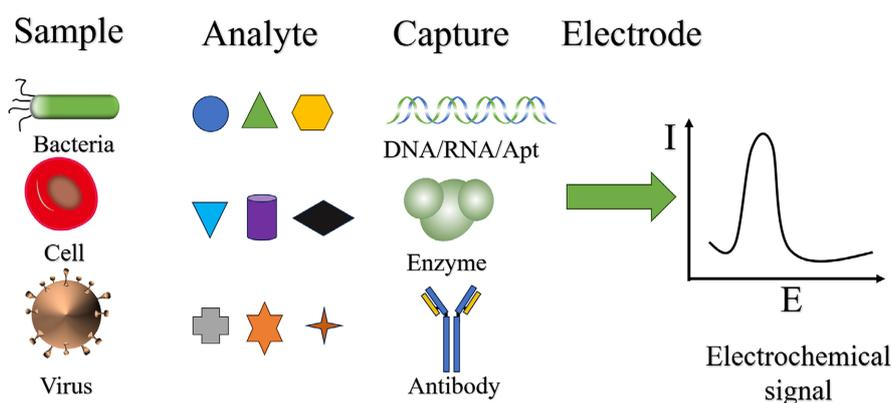
**Figure 1.** The principle of electrochemical biosensor.
