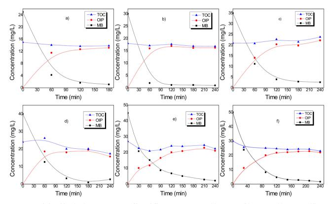
**Figure 6**. Methylene blue (MB) concentration profile at different reaction times: (a) 25 mg/L, (b) 30 mg/L, (c) 35 mg/L, (d) 40 mg/L, (e) 45 mg/L, (f) 50 mg/L showing the reaction behavior based on mass balances and total organic carbon profiles (TOC = total organic carbon, MB = concentration measured by UV-vis spectroscopy, OIP = organic intermediate products).
