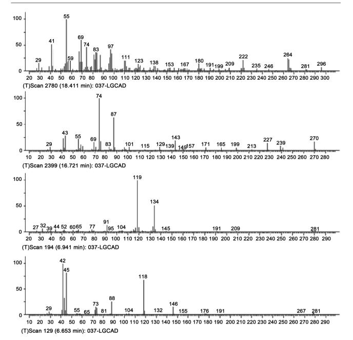
Figure 8. GC-MS spectra of MB degradation at 2 hours of reaction (four peaks are identified with retention times in minutes (a) 18.41; (b) 16.721; (c) 6.941; (d) 6.653).
