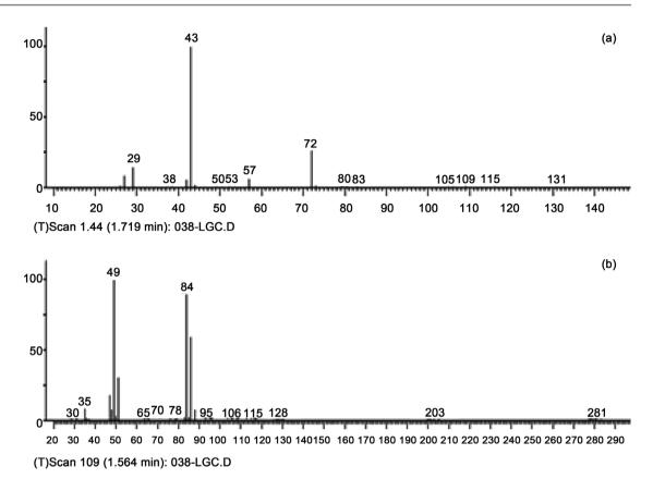
**Figure 9.** GC-MS spectra of the degradation of MB at 4 hours of reaction (2 peaks are identified with retention times in minutes of (a) 1.719 min; (b) 1.5654 min).
