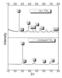
Figure 1. XRD of TiO<sub>2</sub> and Au-TiO<sub>2</sub>.
