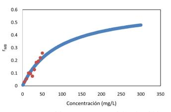
**Figure 7.** Experimental data on Langmuir–Hinshelwood model (LH equation).
