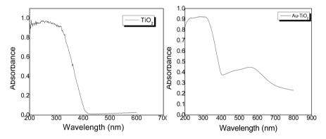
Figure 3. Comparison of the diffuse reflectance profiles of TiO<sub>2</sub> and Au-TiO<sub>2</sub>.
