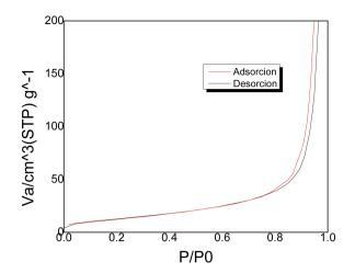
Figure 4. N<sub>2</sub> adsorption-desorption isotherms of Au-TiO<sub>2</sub>.
