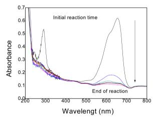
**Figure 5.** Degradation profile of MB of a 10 mg/L MB solution.
