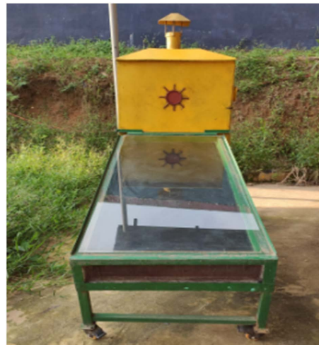
Figure 2. The indirect solar dryer used for the drying experiments.
