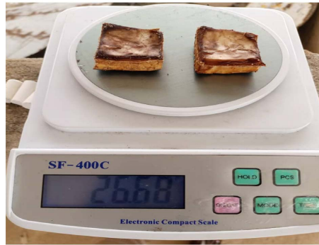
Figure 1. Weighing of samples of shells by an electronic compact scale SF-400C.
