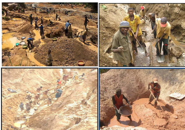
Figure 6. Washing materials, poor recovery. Metals/minerals scavenged by water. Photo credit: Authors.
