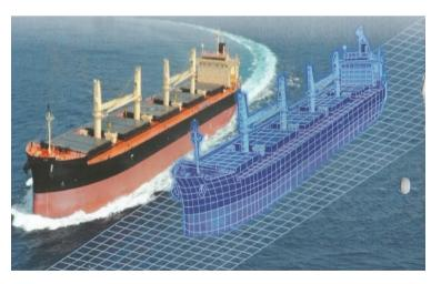
**Figure 1.** The ship and her digital twin. Source: ClassNK (modified) 2019; a digital twin is a reproduction of a ship simulating her movement and operational condition and can make predictions about her.
