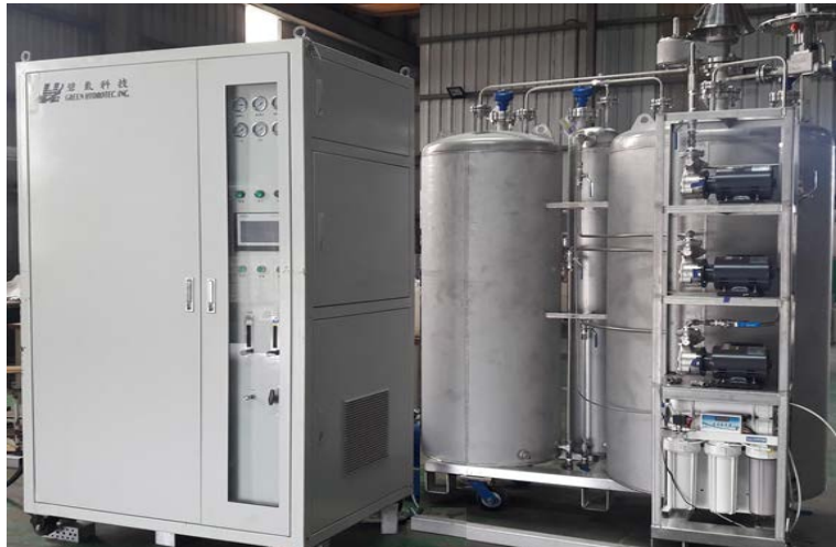
Figure 2. A 40 kg/D onsite hydrogen generator from methanol by Green Hydrotec Inc.
