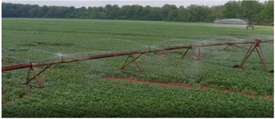
Figure 8. Flying above the pivot and approximately 45 degrees in the direction of the flight path is an efficient protocol for viewing sprinkler anomalies in most situations.
