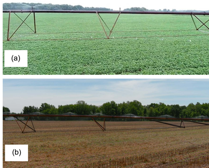
Figure 6. (a) Positioning the UAV at the same height as the pivot span is not useful when there is not sufficient contrast between the water throw and the backdrop. (b) With trees as a backdrop allows to see the water spray patterns.
