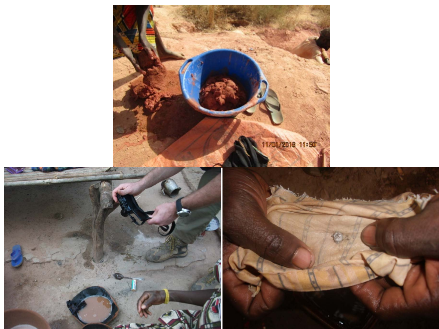
Figure 7. Mercury amalgamation in artisanal mining site.
