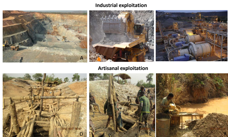
Figure 1. Illustrative images of gold mining in the study area: open industrial pit (A), ore loading (B), ore processing plant (C), artisanal shafts (D), Uptake of ore by artisanal miners (E), artisanal ore washing (F).
