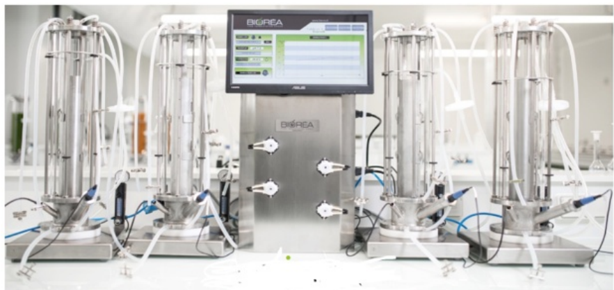
Figure 2. Biological reactor for microbial treatment of petroleum sludge.
