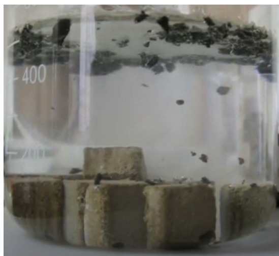
Figure 12. In this experiment, distilled water, QBLOCK™, and small fragments of vegetable carbon were placed, and we observed that the fragments rose and fell in a similar way to when the water was boiled, but in this case, it was due that the fragments of vegetable carbon rose driven by the oxygen bubbles that constantly form inside the QBLOCK™, and then descend attracted by the force of gravity.
