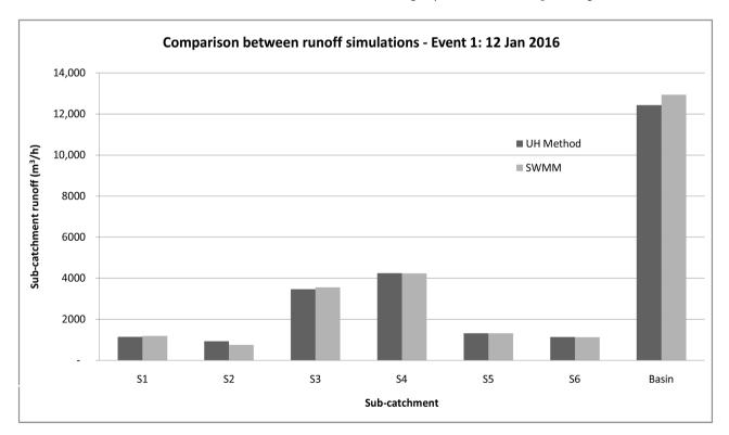
Figure 9. Comparison between mean simulated runoff and observed runoff from discretization using for various sub-catchments of Event 1:12 Jan 2016.
