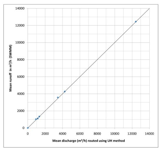
**Figure 8.** Simulated runoff from SWMM and mean of observed runoff from discretization using UH method for Event 1: 12 Jan 2016.
