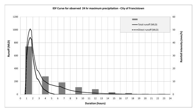
Figure 6. SWMM output of total and direct runoff hydrograph of the main system catchment due to rainfall event 1 of 12 Jan 2016.
