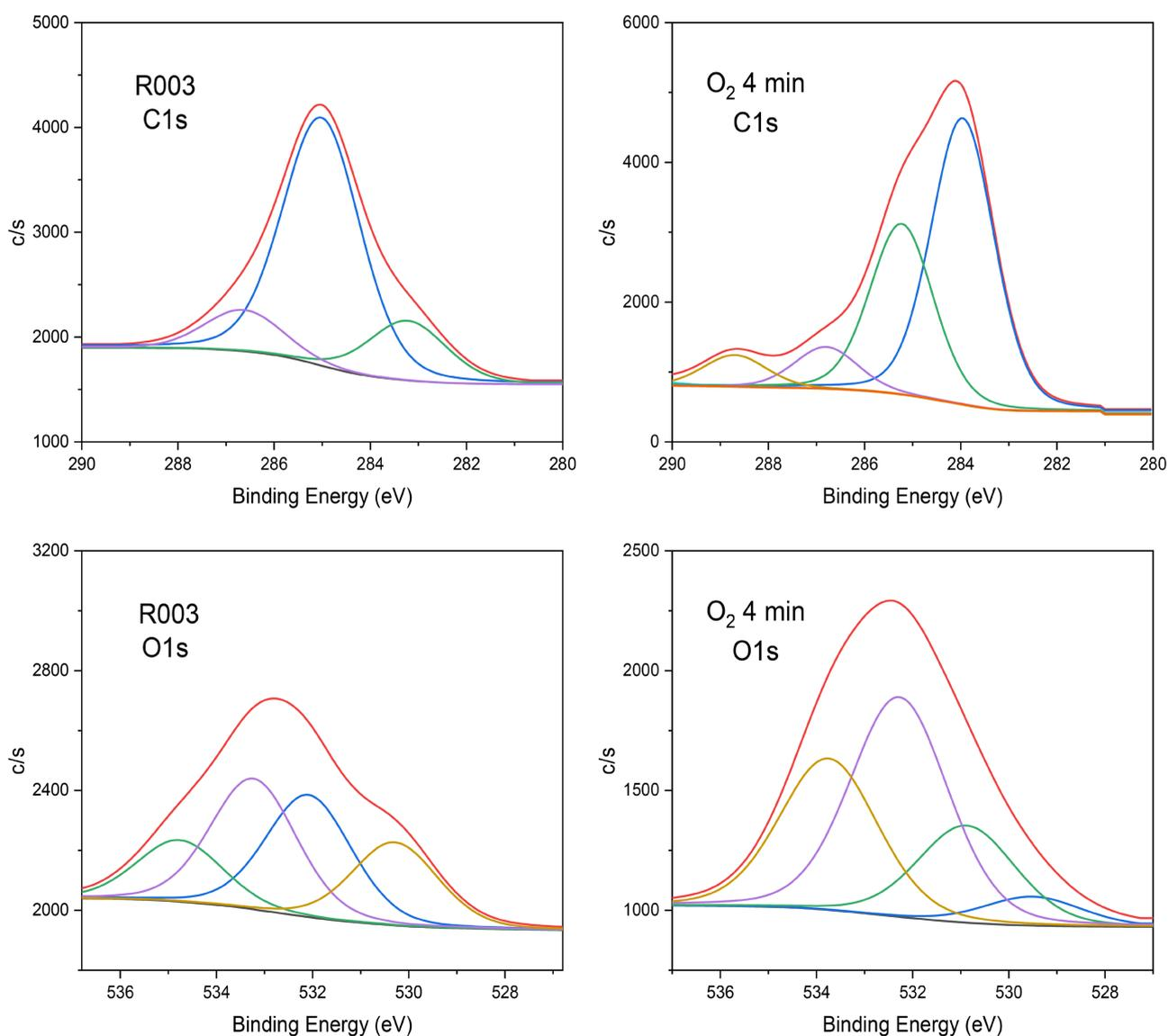
**Figure 6.** XPS data for non-plasma treated AC (top and bottom left) and AC that underwent O<sub>2</sub> plasma treatment for 4 minutes (top and bottom right).
