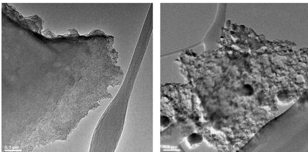
**Figure 5.** TEM images of non-plasma treated AC (left) and O<sub>2</sub> plasma treated AC (right).
