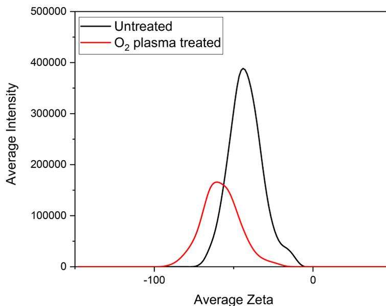
**Figure 7.** Zeta potential data of non-plasma and O<sub>2</sub> plasma treated AC samples.
