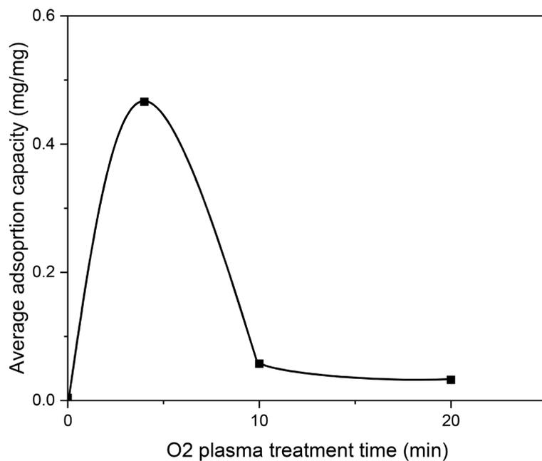
**Figure 2.** Average adsorption capacity of O<sub>2</sub> plasma treated samples with increasing treatment time.
