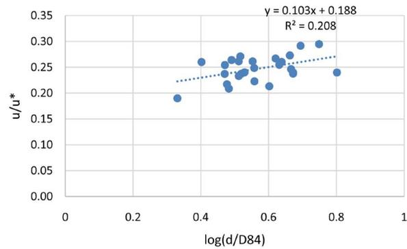
**Figure 6.** Velocity/shear velocity versus  $d/D_{84}$  for six watersheds Maryland coastal plains and piedmont.
