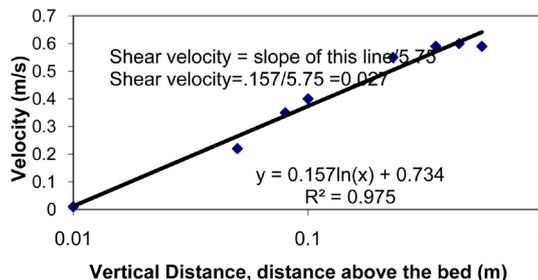
**Figure 2.** Example of velocity profile at a stream station. Velocity was measured in the vertical water column eight times to a height of 0.59 above the bed.
