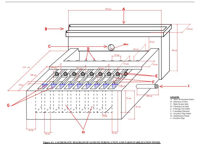
Figure 2. A schematic diagram of on-farm sand filter units and farm stabilisation ponds.
