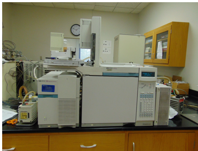
Figure 7. GC-MS used for the pharmaceutical analysis of water samples.
