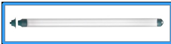
Figure 2. Instrument (Teflon bailer) used for water sample collection.
