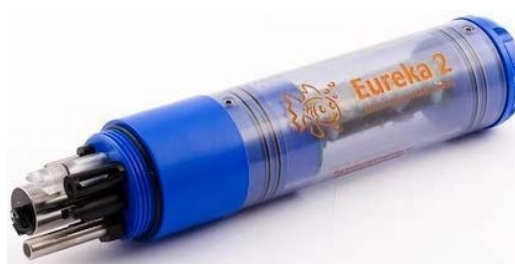
Figure 4. Data logger (Eureka Manta2™) used for in situ monitoring.
