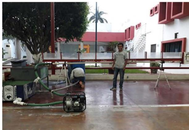
**Figure 1.** Transportable hydraulic channel (VSOCH) of Engineering Faculty of Chiapas State University, Mexico.
