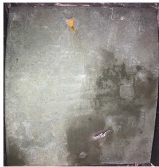
Front of the Greenkote (ELU) Plate After Testing
