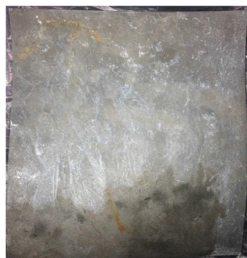
Front of Greenkote (Phosphate) Plate After Testing
