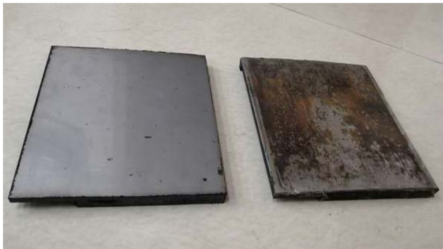
Figure 3. Steel plate without rust and with rust.
