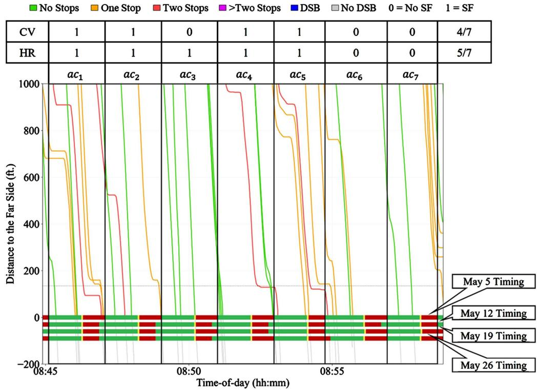
Figure 7. SF evaluation of cycles aggregated by DOW for 8:45-9:00 AM for four Fridays in May 2023.
