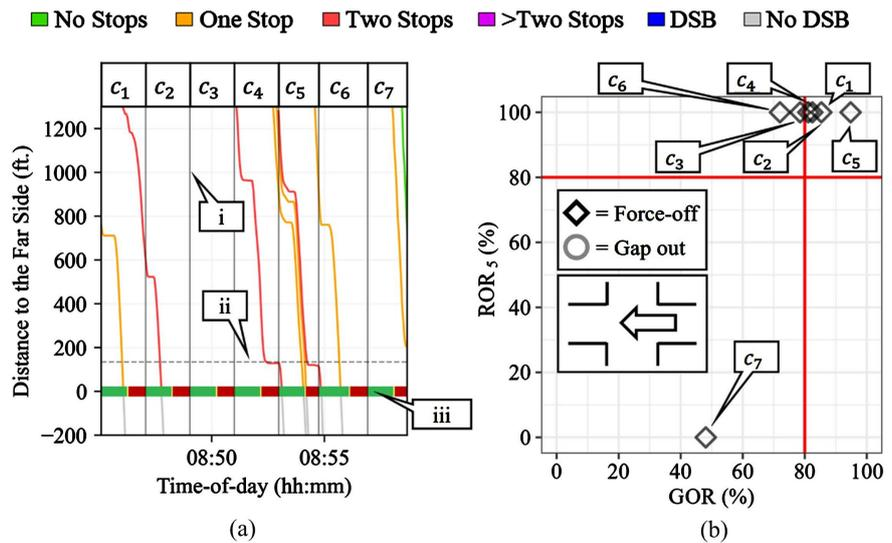
**Figure 5.** CV and high-resolution SF evaluation for 8:45-9:00 AM on Friday May 5<sup>th</sup>, 2023. (a) CV-based TOD PPD; (b) Controller-based  $ROR_5$  vs. GOR.
