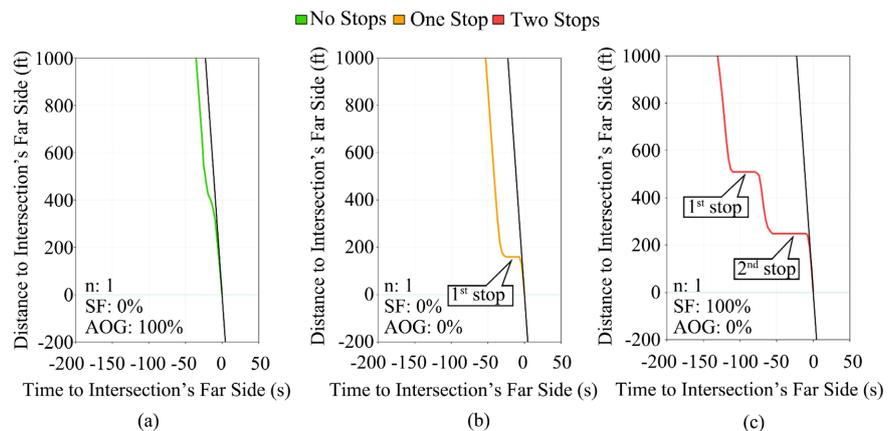
**Figure 3.** PPDs of vehicle trajectories with different number of stops. (a) No stops, AOG; (b) One stop; (c) Two stops, SF.
