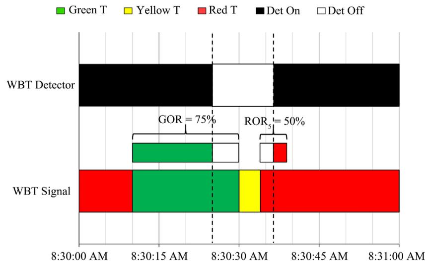
**Figure 2.** Graphical GOR and  $ROR_5$  calculation from signal detector and phase [18].
