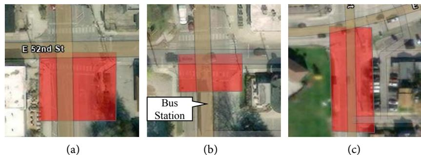
Figure 6. Custom polygon geofences for delay and schedule adherence estimation at intersections. (a) Dedicated bus lane; (b) dedicated bus lane with near-side station; (c) mixed traffic lane.
