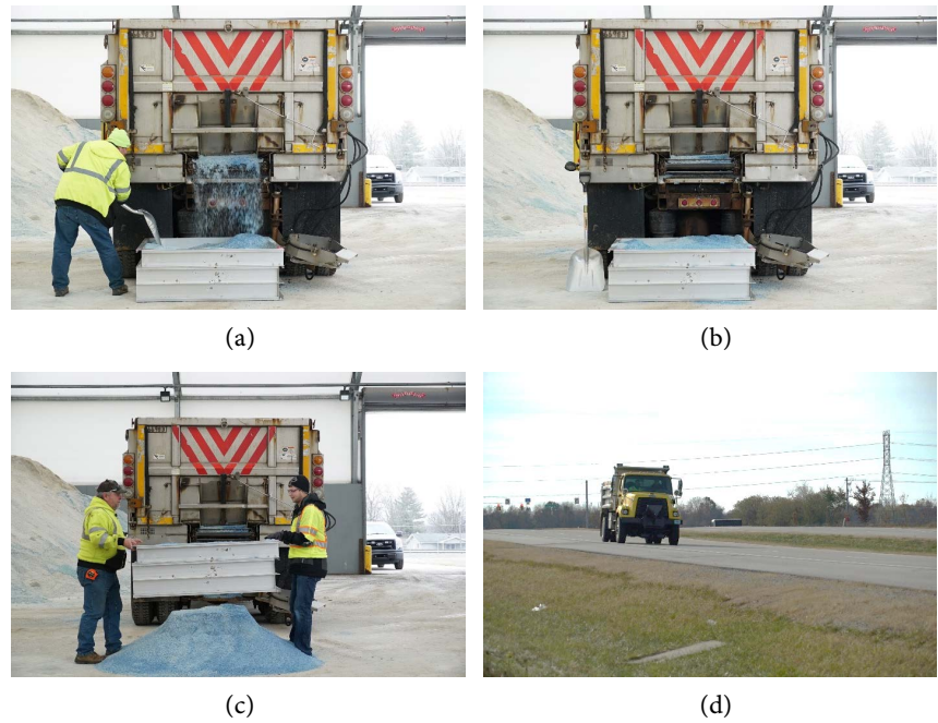
Figure 10. Proposed calibration procedure utilizing the calibration box. (a) Place box under chute and offload into the box; (b) level the box and enter the offload amount in the controller; (c) remove box and return the salt to the inventory; (d) perform the speed calibration.
