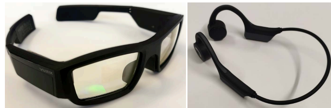
Figure 1. Wearables used in the studies: Vuzix Blade smart glasses and WANFEI bone conduction headphones. Bone conduction headphones do not conceal ambient noise.
