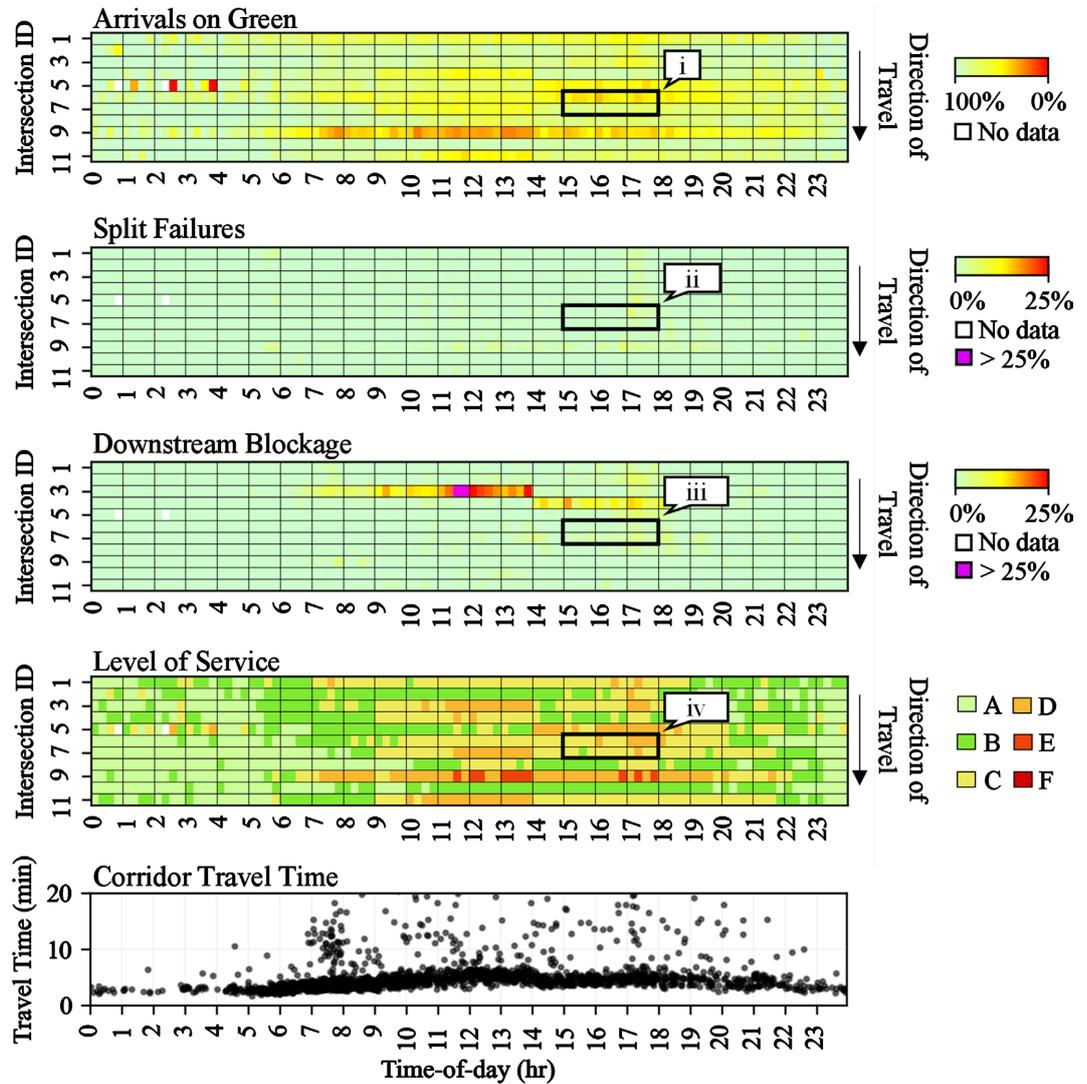
**Figure 3.** Signal performance measures during August 2021 weekdays (after semi-automated adaptive implementation) for vehicle trajectories traveling southbound through.
