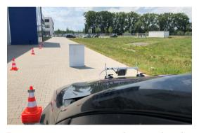
**Figure 8.** Measurement setup to determine the radar cross section of physical test objects.
