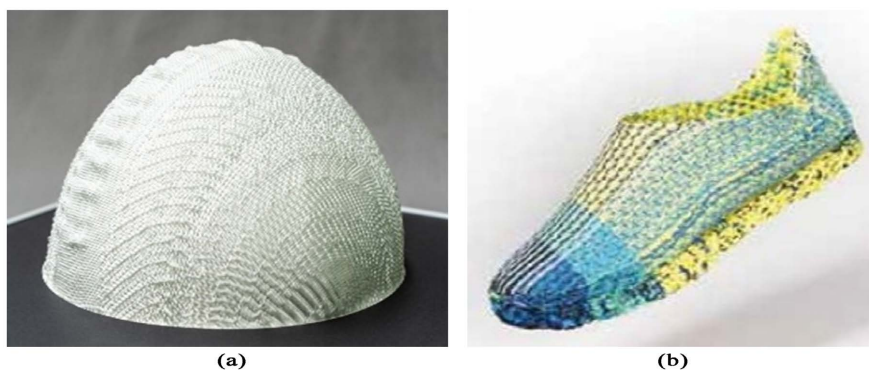
Figure 2. (a) 3D woven preform, (b) woven shoe.
