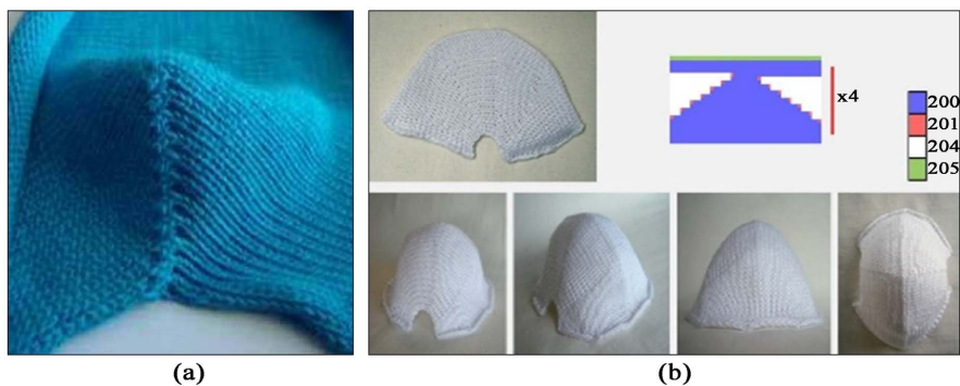
Figure 3. (a) Knitted 3D fabric preform, (b) dome shape formed by suspended stitches, where single jersey knitting = 200, front tuck stitch = 201, no needle selection = 204, cast off (jersey) = 205.
