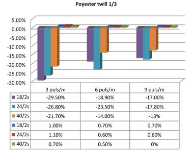
**Figure 8.** Polyester twill 1/3. Effect of both yarn count and jet pulses/min on residual powder % change in rate of air-permeability after pulsing and fabric dust holding capacity.
