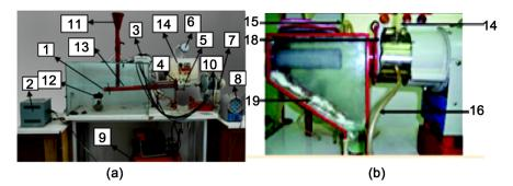
Figure 1. (a): Filtration efficiency apparatus, (b): Close up photo of the testing zone.
