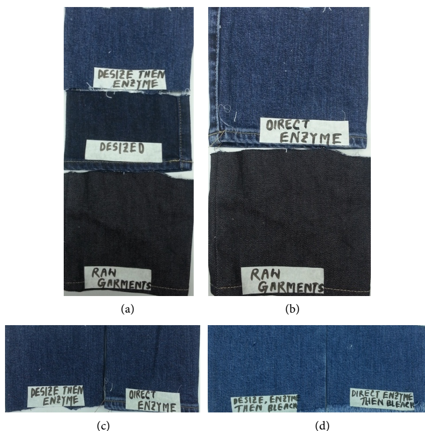
Figure 5. (a) Conventional (raw garment, desize and enzyme); (b) sustainable process (raw garment and enzyme); (c) clear view of color change for enzyme wash (conventional process-with desize and enzyme and sustainable process-without desize, and enzyme); (d) clear view of color change for bleach wash (conventional process-with desize, enzyme and bleach & Sustainable process-direct enzyme, bleach).
