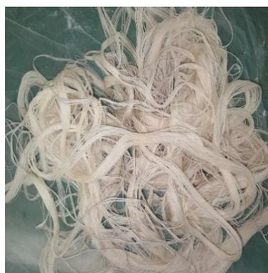
**Figure 4.** Conventionally sized yarn.
