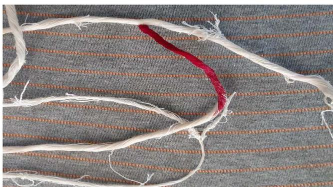
**Figure 8.** Newly sized yarn after absorbency test.
