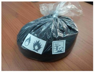
Figure 9. Repackaged vat dye in polythene with warning stickers. Source: Field study, 2020.
