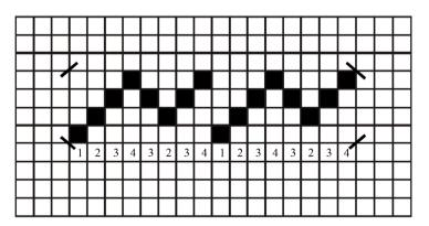
Figure 8. A threading draft for weave plan 6a, 6b, 5c and 6d.
