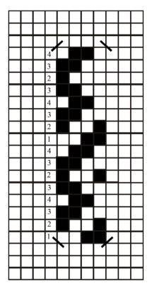
Figure 9. Lifting plan for weave plan 6a.
