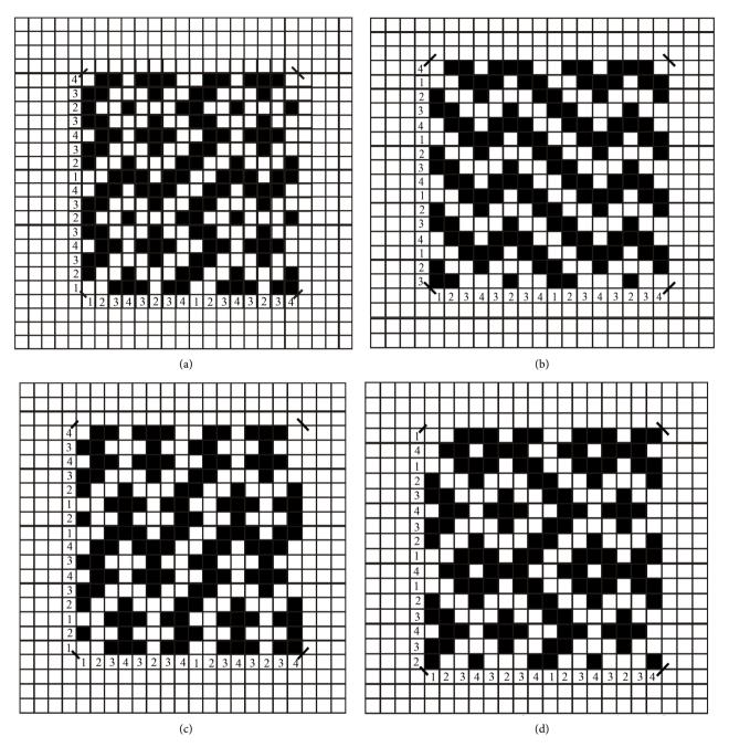
**Figure 6.** (a) Weave plan; (b) Weave plan (variation on weft draft 1); (c) Weave plan (variation on weft draft 2); (d) Weave plan (variation on weft draft 3).
