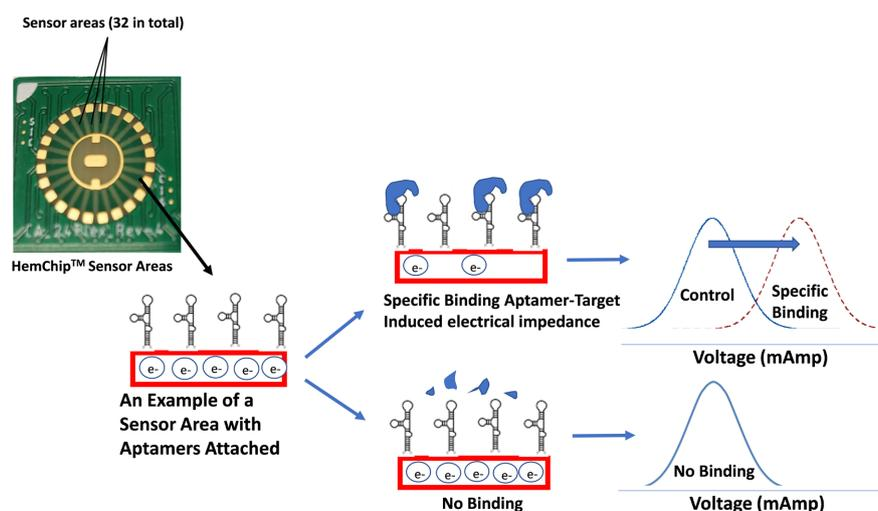
**Figure 2.** Illustration of HemChip™ sensor mechanism. Aptamers were attached to the sensor areas. If there was a specific binding interaction, there will be an electrical impedance resulting in a shift in voltage across the sensor area. Similarly, no electrical output changes occurred if there was no binding event.
