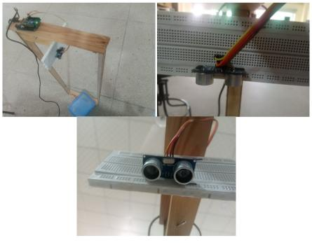
**Figure 1.** Experimental setup for the determination of acceleration due to gravity during free fall motion.
