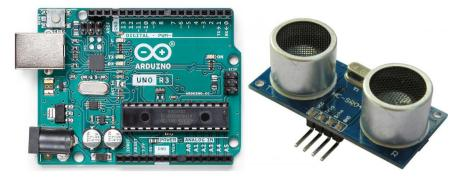
Figure 2. Arduino UNO and HC-SR04 ultrasonic distance sensor [8].
