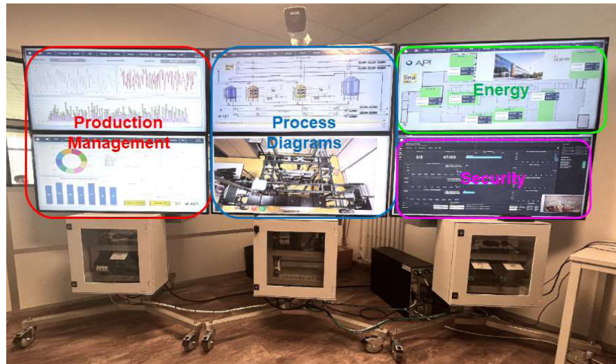
Figure 3. Modular process SKID-MES Lina of API group with process and security screens.
