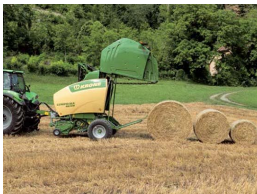
Figure 4. A variable-size chamber baler makes round bales of different diameters.
