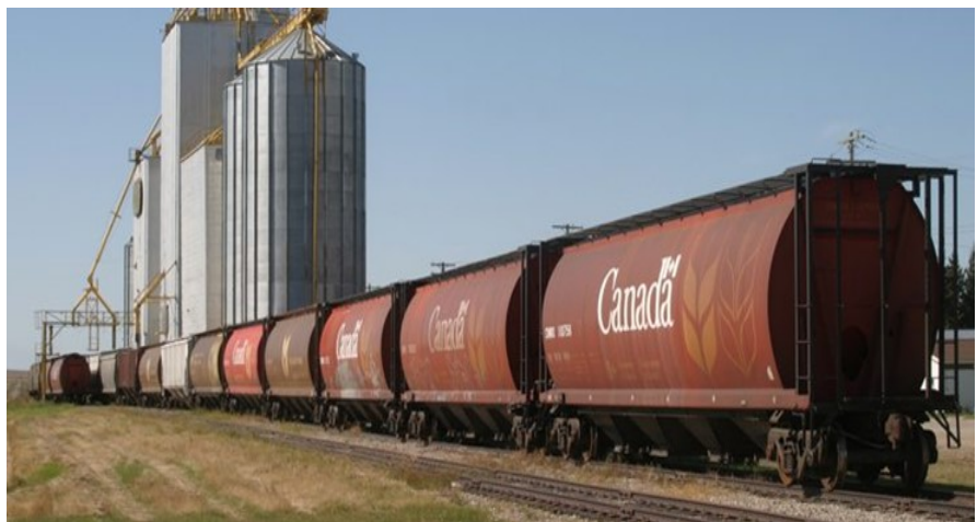
Figure 8. Specially designed grain transport rail cars are used to transport grain in Canada is suitable to transport biomass pellets. Photo Courtesy of Authors.
