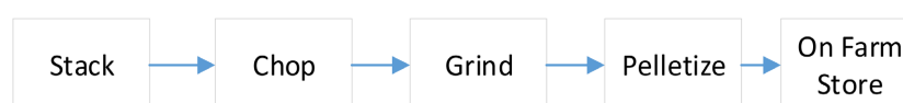
Figure 2. Flow chart showing the sequence of operation involved in preprocessing of biomass.
