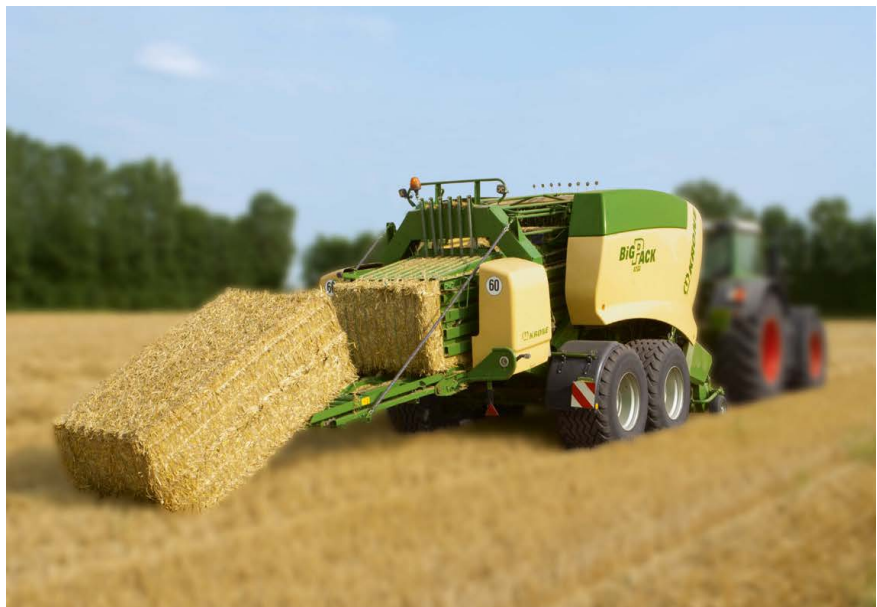
Figure 1. A large square biomass baler (Photo Courtesy of Krone).
