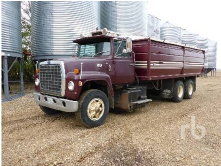
Figure 5. Grain truck that is also suitable for transporting biomass pellets from farm to a central storage site.
