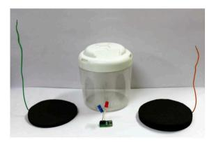
Figure 2. Initial MFC model.
