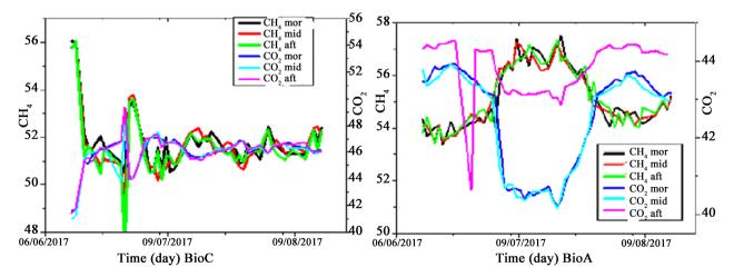
Figure 7. CH<sub>4</sub> and CO<sub>2</sub> content in biogas from the two digesters as a function of time.
