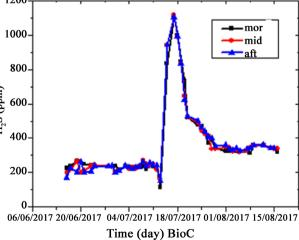
**Figure 9.** Variation of  $H_2S$  in the gas composition of the two digesters.
