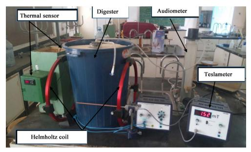
Figure 2. Biodigester with a temperature regulator and teslameter [3].
